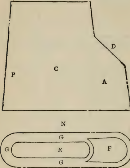
Fig. 135—Represents a side elevation and plan N of a pier of the Potomac aqueduct, arranged with an ice-breaker starling.
